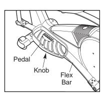
pedals forward or backward to the desired position, and then retighten the knobs. Make sure that both pedals are in the same position.
